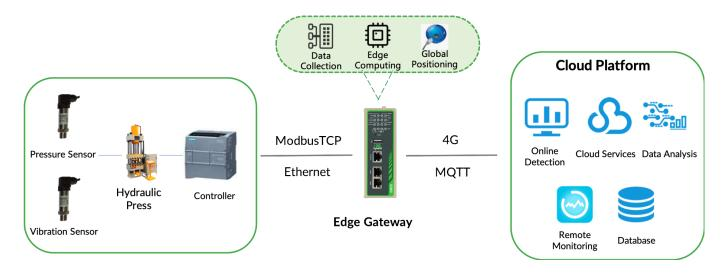
Sensors, hydraulic press, controllers and other devices on site are connected to the edge computing gateway via their respective protocols.
