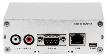
The Instreamer encodes analog audio sources in real time in a configurable format (MP3, CM, G.711, G.722) and streams via TCP, UDP, HTTP, Shoutcast/Icecast and/or Multicast RTP format to configurable destinations.
