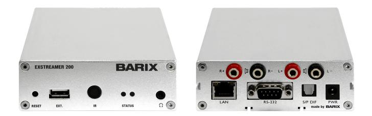
The Exstreamer 20x devices manage and decode IP Audio streams and content, playing out the decoded audio through a built-in amplifier and S/PDIF.
