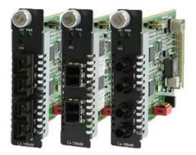
Installed in a high density <u>Perle Media Converter Chassis</u>, Perle's feature rich **C-1000MM Gigabit Fiber to Fiber Media Converter Modules** enable transparent fiber extension of 1000Base-SX multimode fiber to 1000Base-SX multimode or 1000Base-LX/EX/ZX/BX single mode fiber.
