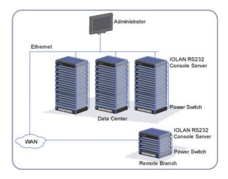
The Perle **RPS**, an intelligent power switch located near the equipment, can remotely power cycle the equipment to restore functionality resulting in decrease risks by reducing mean time to recovery (MTTR).
