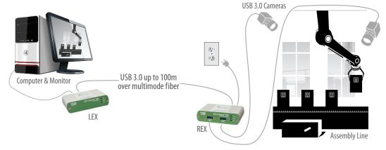
\* Up to 50m with USB 3.0 storage type devices; up to 100m or more is achievable when using USB 3.0 bulk traffic cameras. For Microsoft Kinect applications, please use the Spectra<sup>™</sup> 3001-15 active extension cable.
