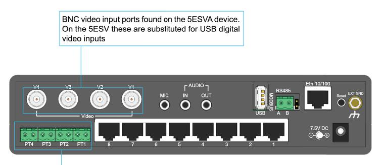
PTZ controller ports, connect with Pelco.D standard PTZ cameras to control the Pan, Tilt and Zoom from the securityProbe web interface.
