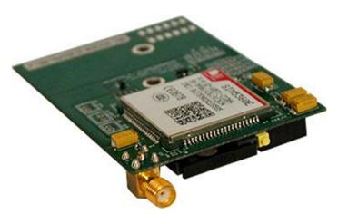
the internal modem is available for all securityProbe and sensorProbe+ platforms. Connect the device to the internet through GSM, GPRS, EDGE, 3G or 4G service.
