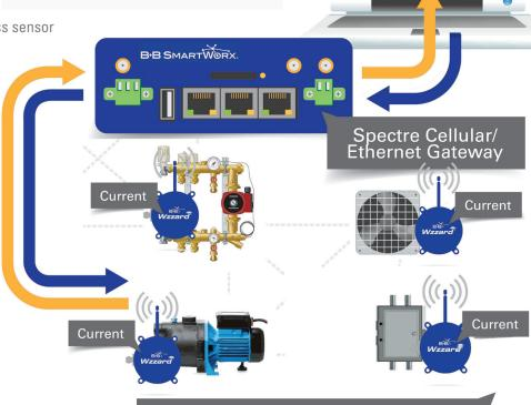
Wzzard™ Intelligent Edge Nodes/ Wireless SmartMesh IP Sensor Network
