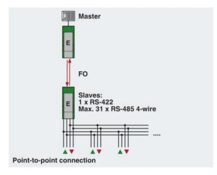
You can network RS-422/RS485 4-wire devices within a star structure as a master/slave network. Depending on the number of star lines required, several PSI-MOS-RS422/FO 850 E Serial to Fiber Converters are connected to TBUS DIN Rail bus systems for voltage and data. This makes up to 10 fiber optic ports available. Cross-wiring for serial data and the supply voltage is provided automatically by the DIN rail connector.
