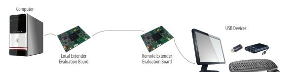
Up to 100m between devices over CAT 6a (or better) cabling and up to 200m with fiber optic cabling
