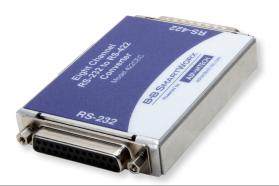
Model 422CEC, 8-channel RS-232 to RS-422 converter, converts unbalanced RS-232 signals to balanced RS-422 signals. The RS-422 Standard uses a balanced voltage digital interface to allow communications of 90K bits per second on cable lengths of 1200 meters (4000 feet). If this baud rate is exceeded the line length will decrease accordingly. Ten receivers can be connected to any one driver for use in multidrop systems.
