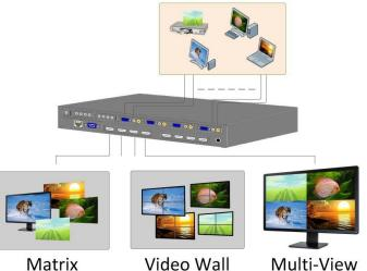
2x2 Picture-Out-Picture or 1+3 Picture-In-Picture Multi-Viewer. The HM-434 matrix switcher can be controlled via panel, IR, RS-232 and TCP/IP.
