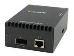
Copper to Fiber conversion is achieved by inserting an XFP fiber transceiver that supports multimode and single-mode fiber, including CWDM/DWDM wavelengths. Copper to copper is achieved by inserting XFP 10Gbase-CX4 transceivers.
