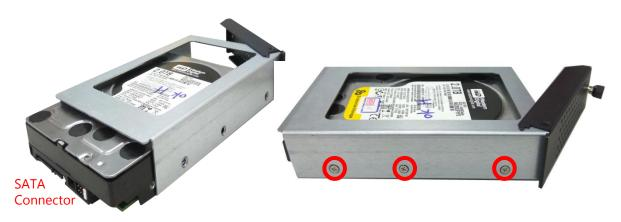
4. Insert the tray into the bay and fasten the screw that fixes the hard disk tray on the front panel.
