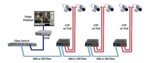
A second option is to have redundant liber links for installations requiring liber facility protection. There is an active fiber port and a protection fiber port that can support a fiber failure switchover of less than 50 milliseconds. The Hi-PoE media converter supplies power to the camera, and has power protection from an Uninterruptible Power Supply (UPS) battery back-up. In the event of a fiber cut and a loss of power, the camera continues to send data on the protection link.
