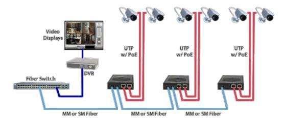
A second option is to have redundant fiber links for installations requiring fiber facility protection. There is an active fiber port and a protection fiber port that can support a fiber failure switchover of less than 50 milliseconds. The Hi-PoE media converter supplies power to the camera, and has power protection from an Uninterruptible Power Supply (UPS) battery back-up. In the event of a fiber cut and a loss of power,
