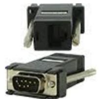
DBA0021C 8pck - 8 pack of #04007050 RJ45F to DB9M (DTE) crossover adapter for IOLAN.
