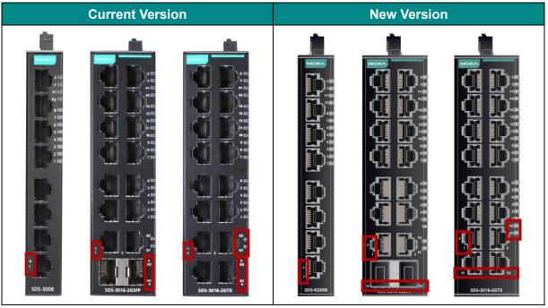
• The new product versions will be embedded with the new firmware version v3.0, with additional functions, including Fiber Check and Trusted Access. Firmware version v3.0 is compatible with both current and new hardware version products, but firmware version v2.2 or before is not compatible with the new hardware product versions.
