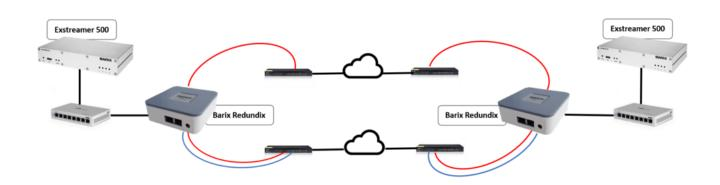
Redundix by Barix is a solution that improves the quality of an RTP stream link using two mechanisms. The first is time-diverse routing, where the same audio stream is sent twice over the same link, immediately on encoding, and also time-delayed. The second is path divergent routing, where two streams are sent using separate networks.
