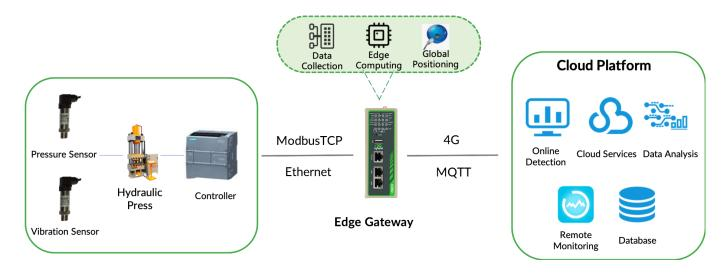
Sensors, hydraulic press, controllers and other devices on site are connected to the edge computing gateway via their respective protocols.
