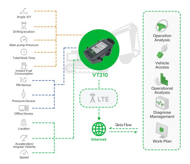
Featuring extensive I/O, standard protocols for communications and vehicle diagnostics, the VT310 can be connected to multiple peripherals on board (e.g. alarms, sensors, switches, controllers, etc.), conducts various functions including real-time engine diagnostics, anti-theft, days in use/on site, maintenance, etc.
