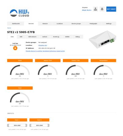
And trigger an alert sent directly from the portal. Understandably, if the power goes out - no SMTP destination would be able to receive an alert because it couldn't be sent. When the device comes back on, its status in the portal changes within a
